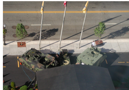
A top view of the displayed combat vehicles at the 2004 conference. From left to right, they are the 1064 Mortar Carrier, Gator adapted for transporting M120 Mortar Systems and the M577 Fire Direction Control Vehicle.
